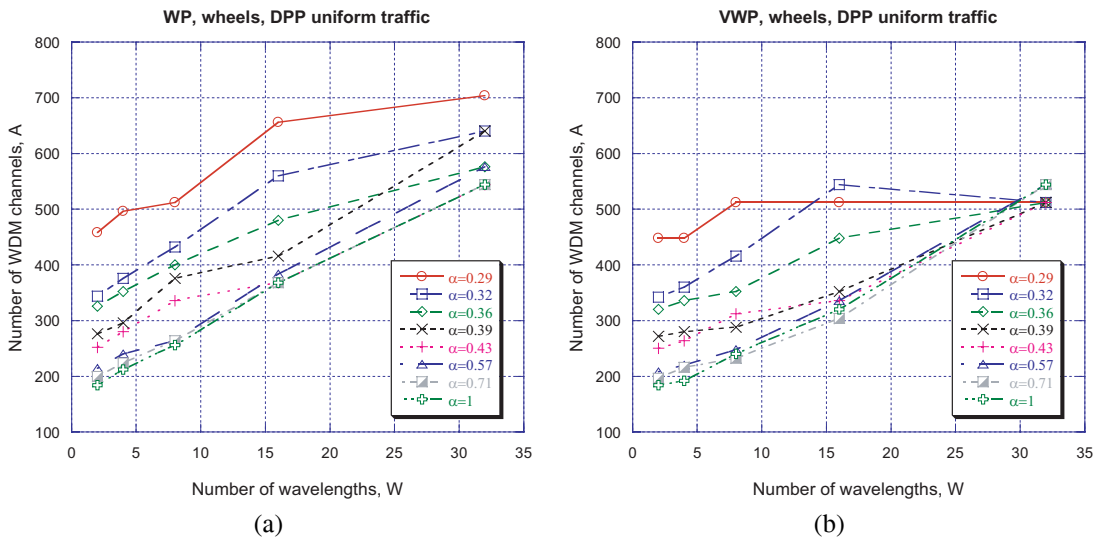
Fig. 5. Number of installed WDM channels A as a function of W for DPP uniform traffic: WP “wheel” networks (a); VWP “wheel” networks (b).
